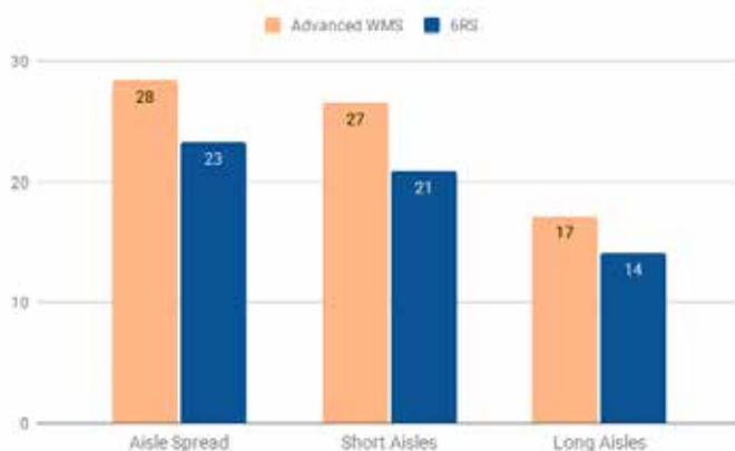
Figure 1. To complete the same work, on average, Chucks traveled down 22% fewer aisles and guided pickers to an 18% tighter grouping than the WMS.
